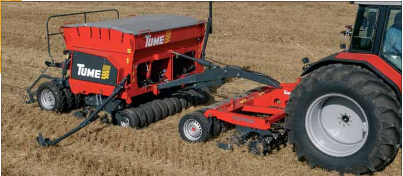
The drawbar can be mounted in the upper position for applications such as CultiPack combination.
