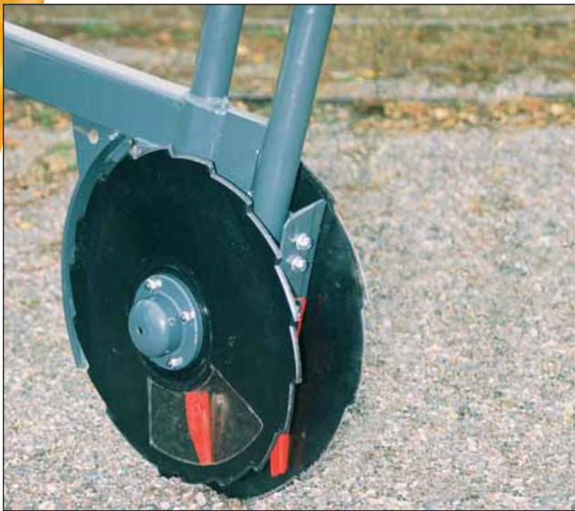
The Nova Combi's ELMIA-award-winning double-disc coulters.
